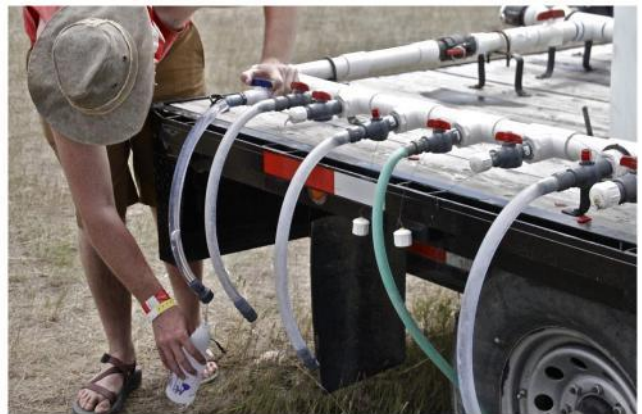
A water tank mounted on a trailer is used to provide potable water for drinking and spray bottles.
